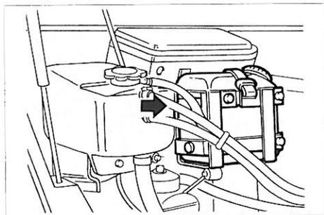
Fig. 67 – Serbatoio lavacrystallo
